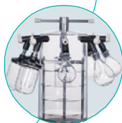
D: Top-Press Multi-Manifolds (TPMM)
