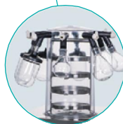
C: Ordinary Multi-Manifolds (OMM)
