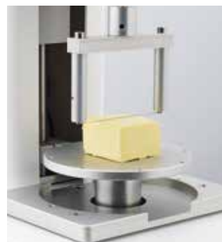
TX-WSF : WIRE SHEAR FIXTURE (Ref. 130076R) Accessory to measure consistency of product as Butter or Cheese.
