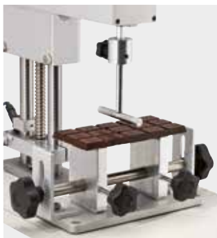
TX-TPBF : 3 POINTS BEND FIXTURE (Ref. 130091R) Breaking strength, Friability, Springiness.
